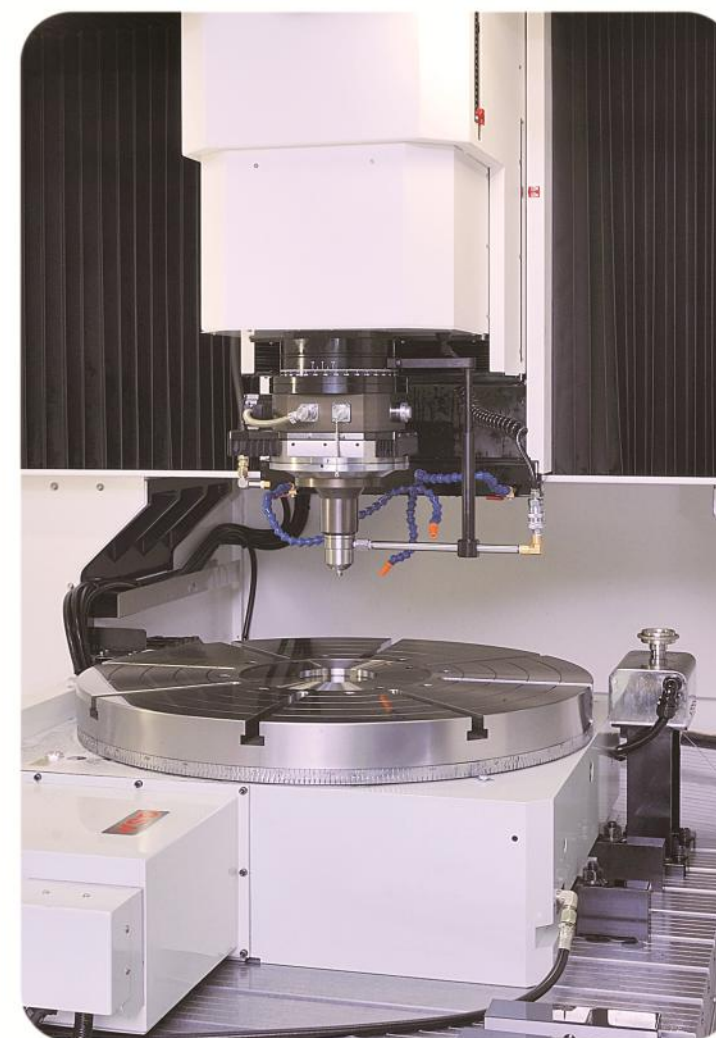
增加第四軸之應用 Additional fourth axis install to use
