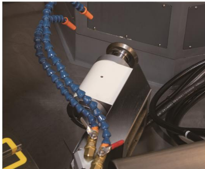
修砂器90度起降 90 degree rotation dresser
